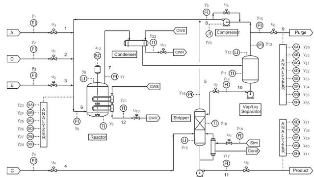
Fig. 2: Production scheme of the Tennessee Eastman process.
